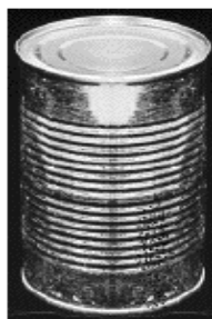
Pitted rust or leaking
